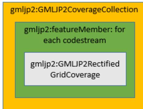
**Figure D.2 – GML structure**
