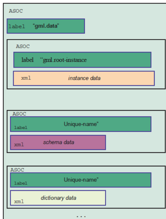
Figure D.1 - GML box structure
