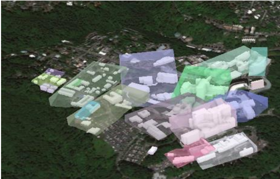
Figure 5 - 3D objects enclosed in an oriented bounding box (OBB).
