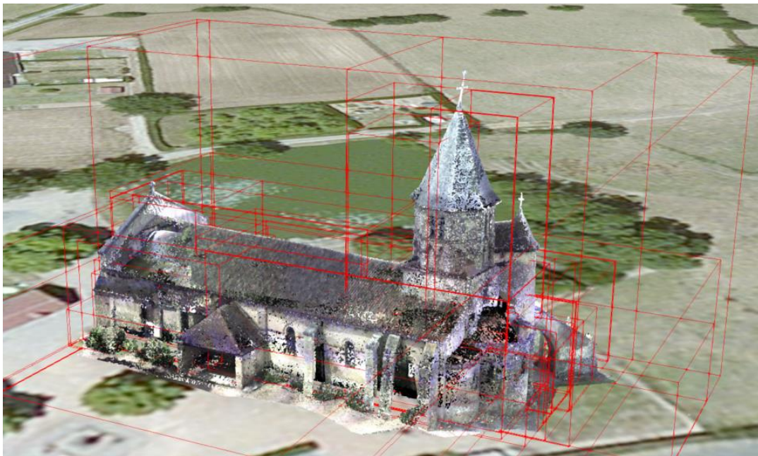
Figure 6 - Tile's division of a point cloud tileset.
