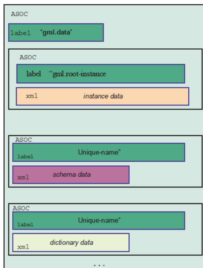
Figure D.1 - GML box structure
