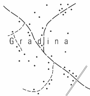
Figure 25. Labelling of a populated area with widely scattered buildings
