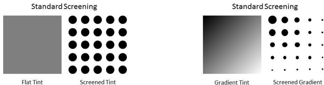
Figure 10: Halftone dots standard screening
