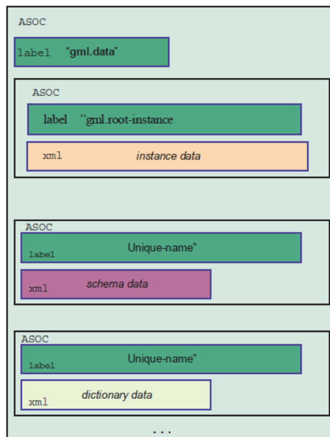
Figure D.1 - GML box structure
