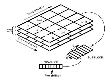
Figure 5-6 Raster Logical Structure (Conventional Orientation)
