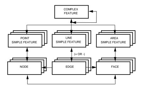
Figure 5-2b Exchange Structure Schema (Optional two-way pointers)
