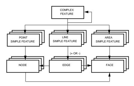
Figure 5-2a Exchange Structure Schema (Mandatory one-way pointers)
