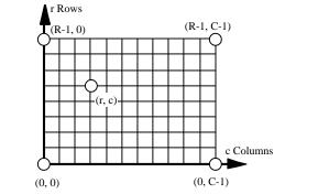
Figure 5-8 Matrix Coordinate System (Conventional)
