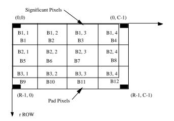
Figure 5-7 A Blocked, Padded Image (Display Orientation)
