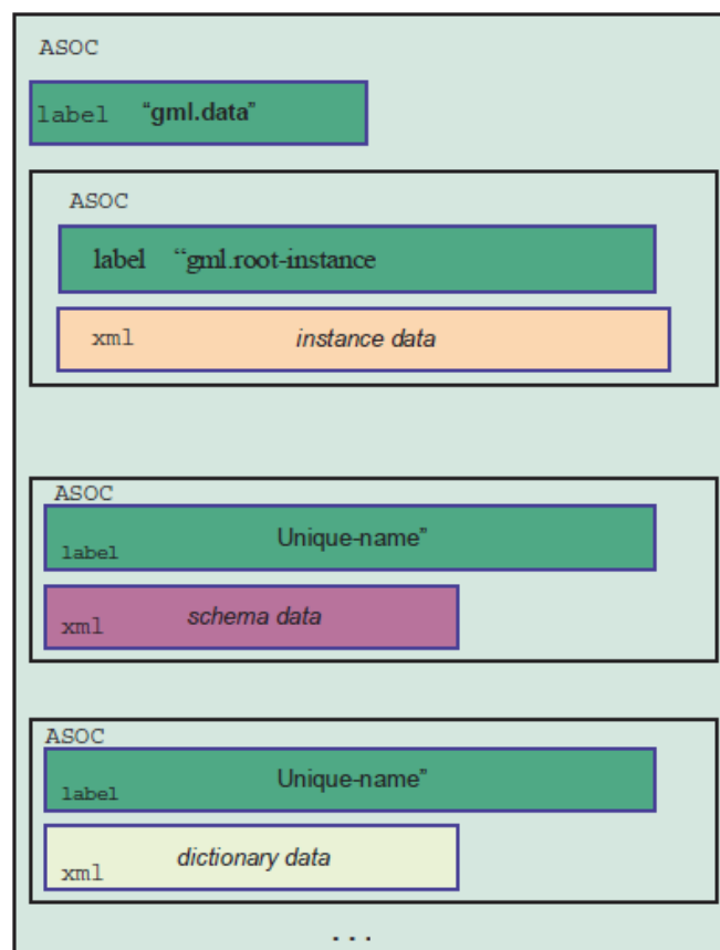
Figure D.1 - GML box structure
