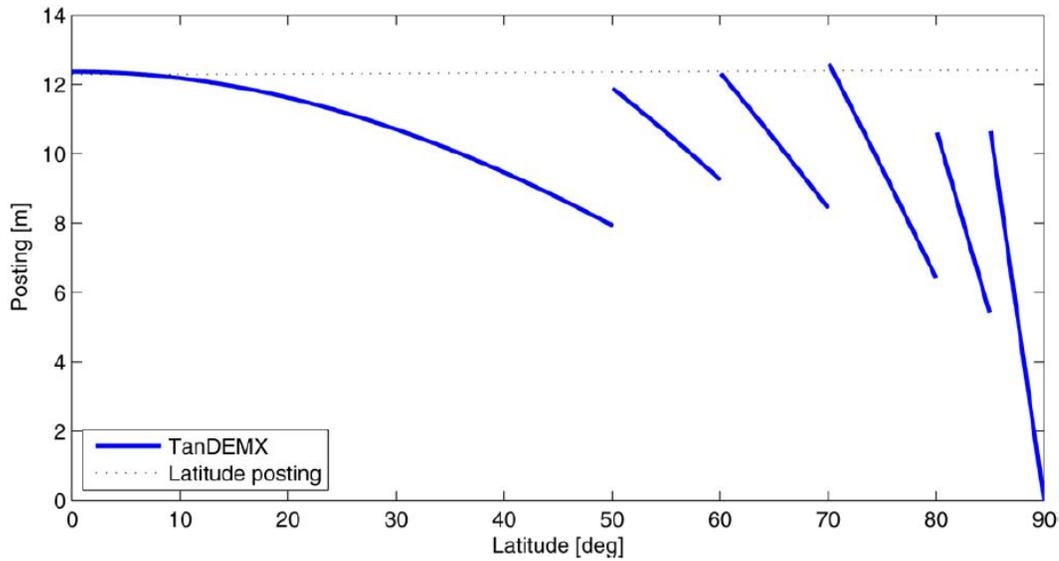
**Figure 4 – Longitudinal posting as a function of latitude**
